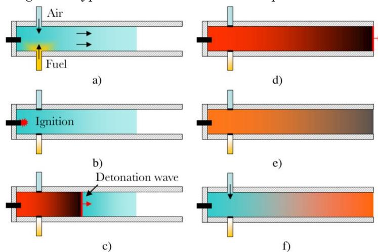
**Figure 3.** Work cycle of PDE
