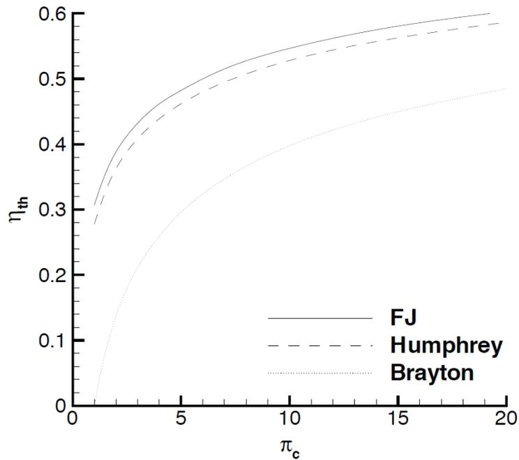
**Figure 4.** Thermodynamic energy conversion coefficient at various compression rates in compressor
