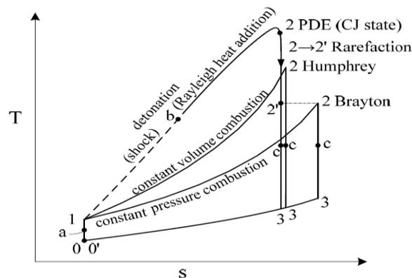
**Figure 2.** Comparison of different thermodynamic cycles in coordinates temperature (T) - entropy (S) (Tangirala & Dean, 2007). (CJ) - Chapmen-Jouguet detonation
