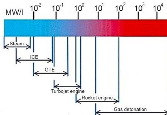
**Figure 1.** Comparison of power, megawatt (MW) per liter (l) of modern heat engines
