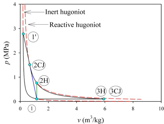
**Figure 6.** Diagram pressure( $p$ ) - specific volume ( $v$ ) for Humphrey (H), Fickett - Jacobs (CJ) cycles and real detonation engine
