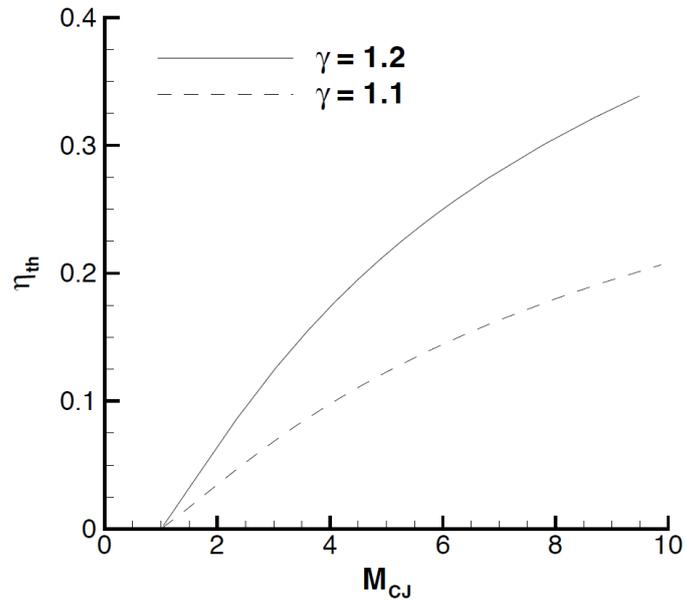
**Figure 5.** A thermodynamic energy convection coefficient at various Mach numbers of Chapman-Jouguet detonation wave's propagation
