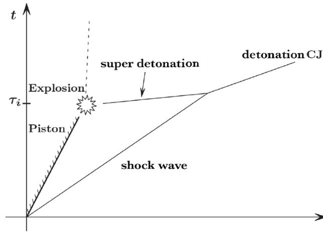
**Figure 9.** Transition of spherical detonation to Chapman-Jouguet mode.  $\tau_i$  - the moment of explosion
