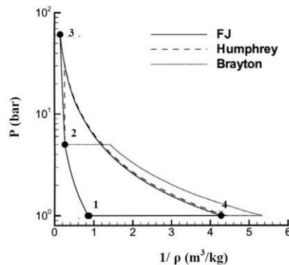
**Figure 1.** Thermodynamic cycles: FJ - Fickett-Jacobs detonative combustion cycle on stationary CJ detonation mode, Humphrey - combustion at constant volume, Brayton - combustion at constant pressure
