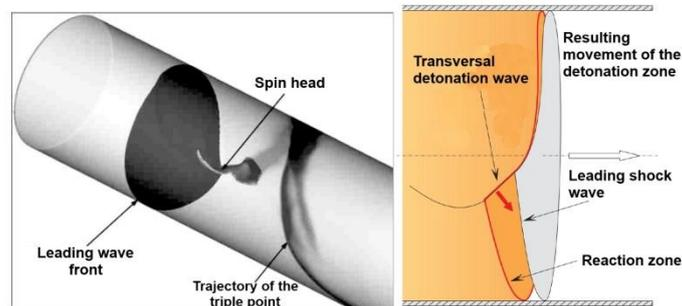
**Figure 3.** The structure of spin detonation in channel
