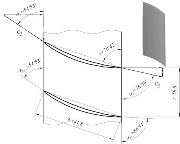
**Figure 2.** Cascaded airfoils of a VGV's first blade in medium section, 3D model of a blade
