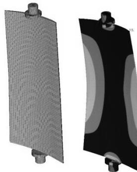
**Figure 6.** FEM-model of a VGV blade and distribution of tensions: maximal tensions 238 MPa, and 106 MPa on the airfoil
