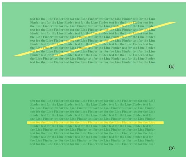
**Figure 5.** Sketches of the light color line formed in the device. a) Double parallel lines that may form before adjusting the device, b) Highlighted main line, as observed after adjusting the device
